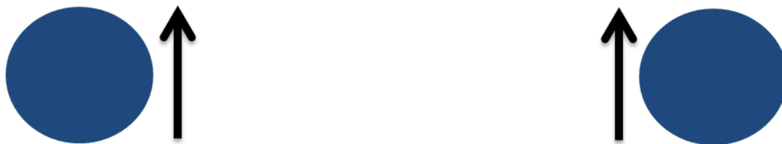
Figure 3-3: Indirect exchange coupling takes place due to larger interatomic distance between the adjacent atoms leads to a parallel alignment
